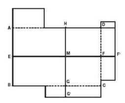
In corridors and small spaces, it may be simpler to work lengthwise from one end, using the centre line as a guide. The centre line is drawn as follows: a chalk line is snapped from centre of wall A-B (=E) to the centre of wall C-D (=F). The centre of line E-F is found (M). Draw a perpendicular line through M using the 3:4:5 method to establish G-H (Figure A).
